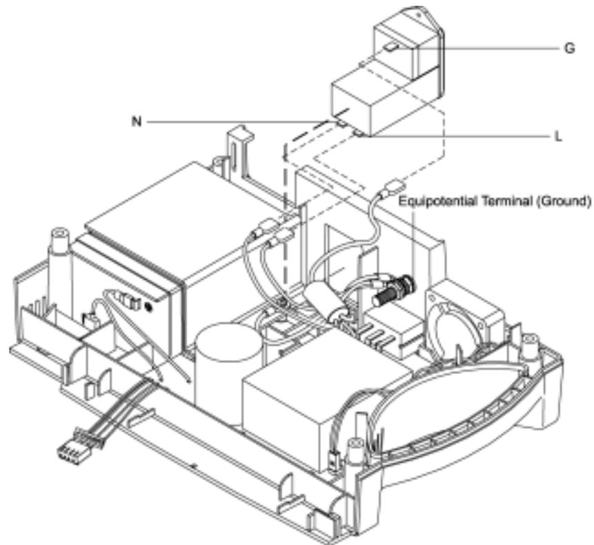
**Figure 8: Power Entry Module**
