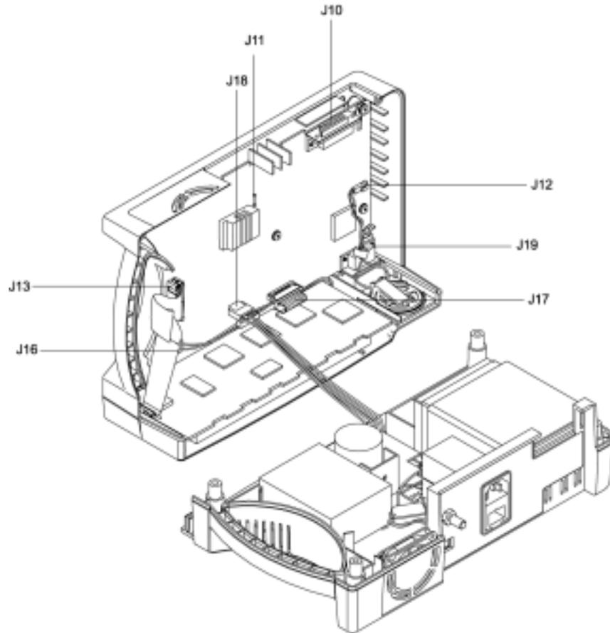
**Figure 6: Separating Case Halves**
