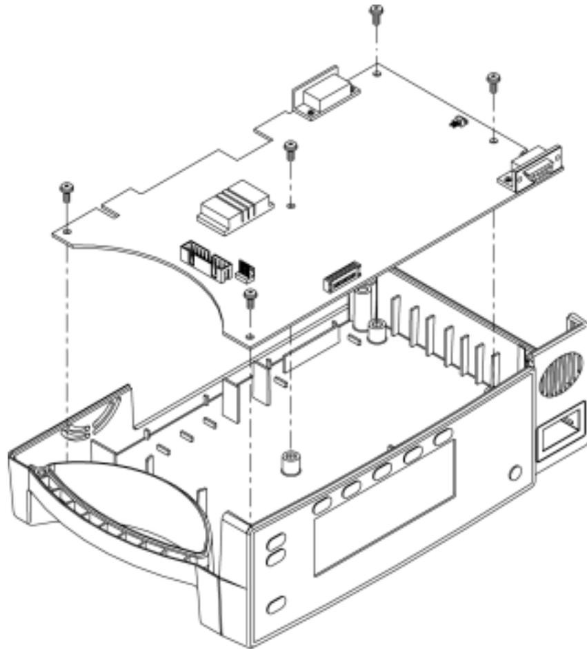
**Figure 12: User Interface PCB**
