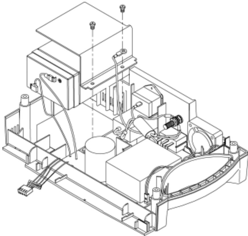
**Figure 7: Removing the Battery**
