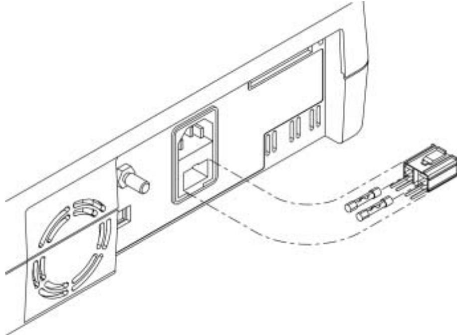
**Figure 4: Fuse Removal**
